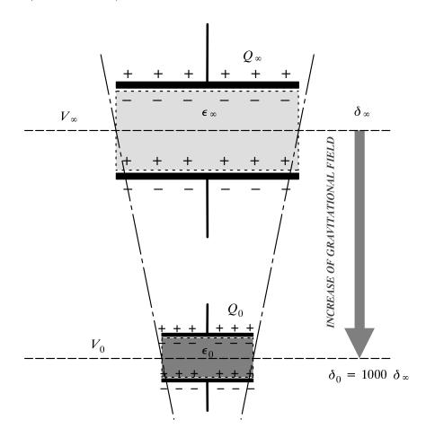
Figure 1: A capacitor "plunged" into a gravitational field
